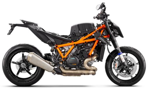
The frame also received a few minor tweaks to compensate for the updated engine, gearbox and larger fuel tank. The frame uses the engine as a means to increase torsional rigidity, making the KTM 1390 SUPER DUKE R EVO extremely precise. This allows for an effortless, confidence-inspiring riding position, translating into an ultimately faster ride. This is achieved by maximizing the feedback from the chassis and the front tire. The frame also makes use of thick-diameter tubes with thin walls for o
